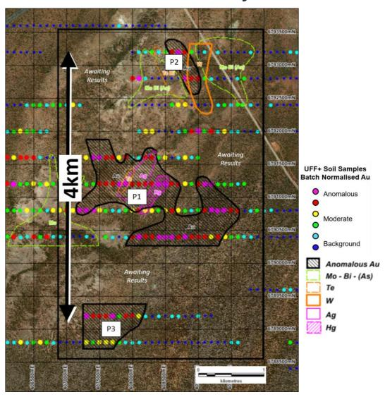
**Figure 2**: East Well Anomaly: Schematic plan showing the >4km long UFF+ gold soil anomaly, defined by the distribution of batch normalised gold results. Coherent zones of coincident multi-element geochemical anomalism have been highlighted. These zones have been prioritised and scheduled for field validation.
