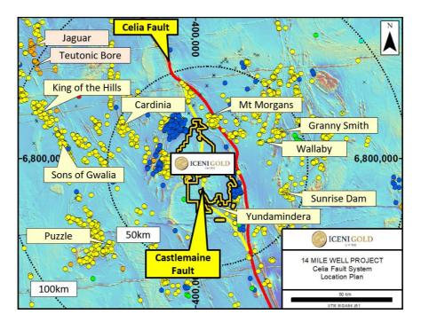
**Figure 4:** The **Celia Fault zone** passes along the eastern margin of the 14 Mile Well project, while a splay off this fault, the **Castlemaine Fault**, passes through the centre of the project area. In the **Claypan a**rea the **Celia Fault** has a significant change in orientation where it interacts with the Castlemaine Fault.
