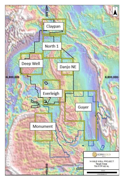
**Figure 2:** 14 Mile Well project area, showing the seven key target areas. Diamond drilling is underway within the **Claypan** target area designed to test beneath surface geochemical and geophysical anomalies. Image is Total Magnetic Intensity (TMI) Reduced to Pole (RTP) (after GSWA).
