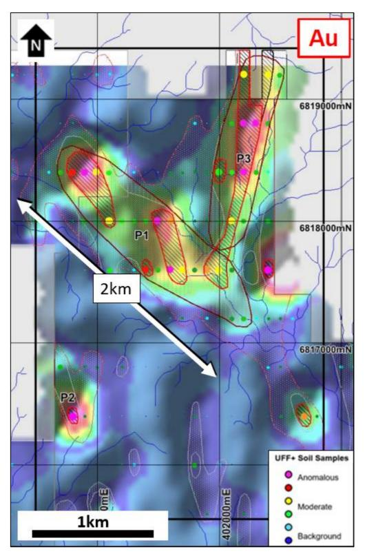
**Figure 5:** The UFF+ gold anomaly 14UF014 at **Claypan** has a priority 1 zone that is 2km long, this priority 1 zone is coincident with the sub-cropping SCT/BIF unit.
