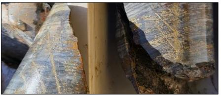
Figure 1: BIF in FMDD0039 ~109m, the pyrite displays a telegraph texture.
