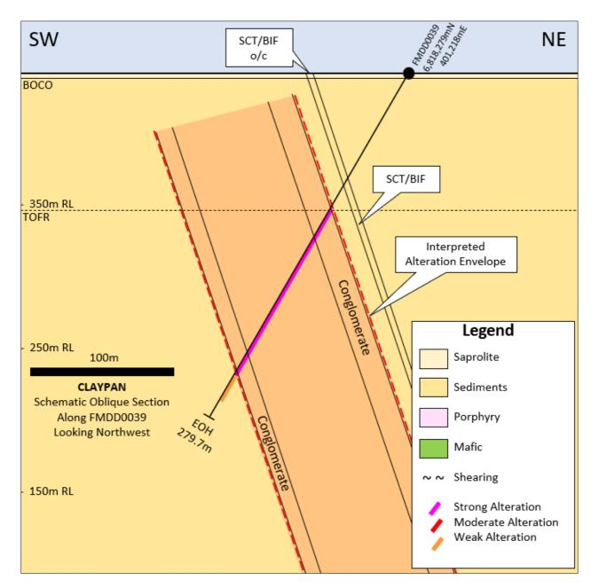
**Figure 5:** Oblique schematic section along the trace of hole FMDD0039, looking northwest. The strong to intense alteration envelope is focussed along the coarser clastic sediments/volcaniclastics.
