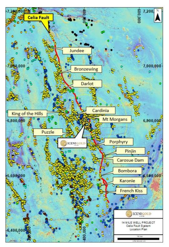
Figure 3: The Celia Fault is a major crustal structure know to extend across the Yilgarn Craton for ~700km. Significant gold deposits spatially related to the Celia Fault include: Jundee, Bronzewing, Darlot, Mt Morgans, Carosue Dam and Karonie.
