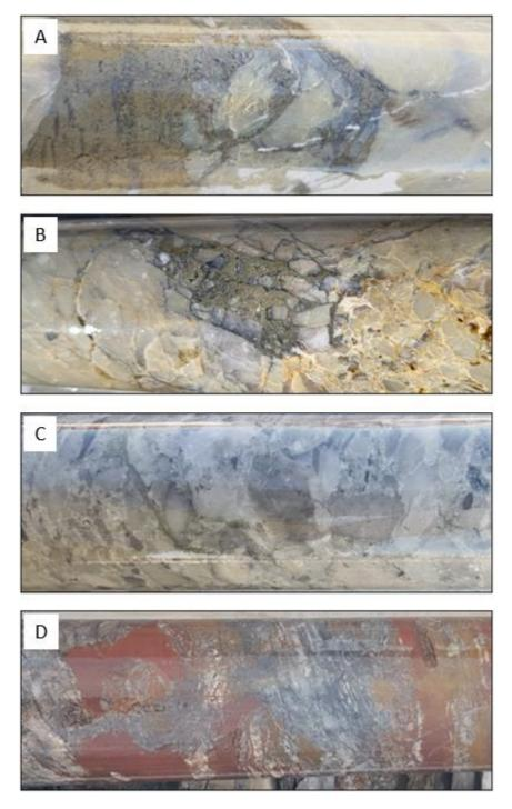
Figure 6: Observed alteration in diamond drilling beneath UFF+ Au anomaly 14UF014 at Claypan.
