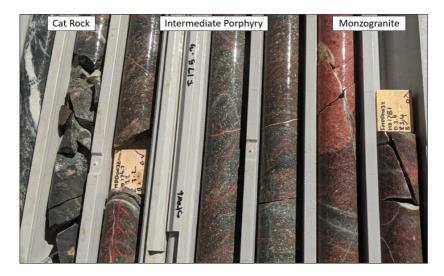
**Figure 7:** FMDD0032 ~ 175m Hematite-silica altered intermediate porphyry that cuts the Danjo Monzogranite and exploits the adjacent cat-rock contact.
