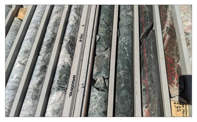
**Figure 8:** FMDD0032 ~190m. Example of alteration and structural complexity within the Castlemaine Fault. Hematite alteration and quartz veining within the Danjo Monzogranite is apparent at the top of the image. In the centre of the image the entire rock mass is brecciated and silica flooded. In the lower part of the image the rock is overwhelmed by multiple generations of quartz and carbonate veins.
