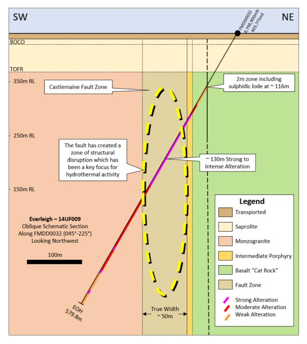
Figure 4: Oblique schematic section along the trace of the hole FMDD0023, through the Castlemaine Fault.
