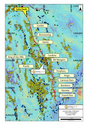
**Figure 5:** The **Celia Fault** is a major crustal structure known to extend across the **Yilgarn Craton** for ~700km. Significant gold deposits spatially related to this fault include: **Jundee, Bronzewing**, **Darlot**, **Mt Morgans, Carosue Dam** and **Karonie**. Background image TMI RTP (after GSWA).
