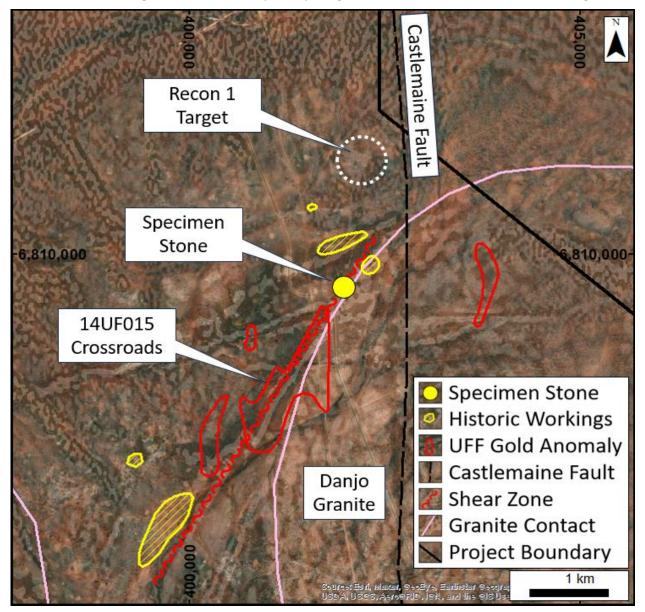
**Figure 5:** Location of the gold in specimen stone relative to the key structural and geochemical characteristics of the Crossroads target (background image is composite magnetics VD1-Airphoto).
