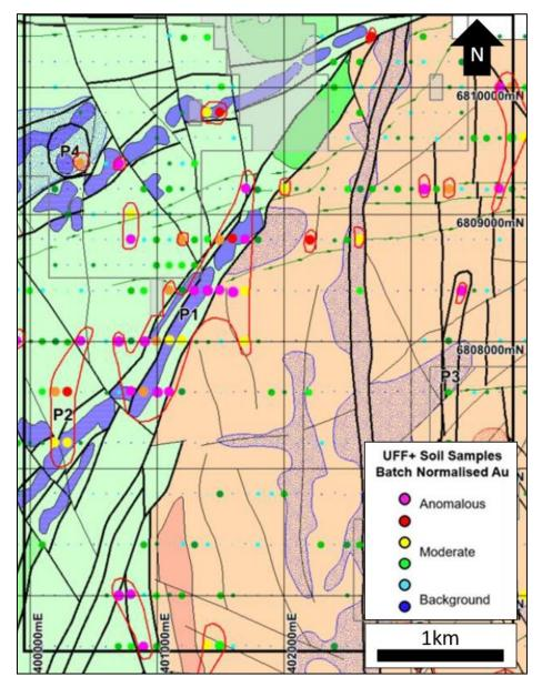
Figure 4: Anomaly 14UF015 is a Au-Te-W anomaly associated with a northeast trending magnetic ridge at North1. (ASX release 31 August 2022)
