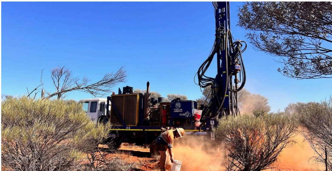
Figure 1. Air core drilling at Guyer.
