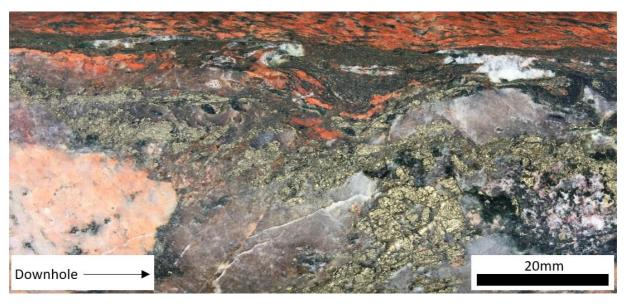
**Figure 4:** Alteration zone in FMDD0002 at ~79m downhole; hematite altered granodiorite hosting quartz veining with tourmaline and pyrite; beneath historic hole KOW014, at Deep Well.
