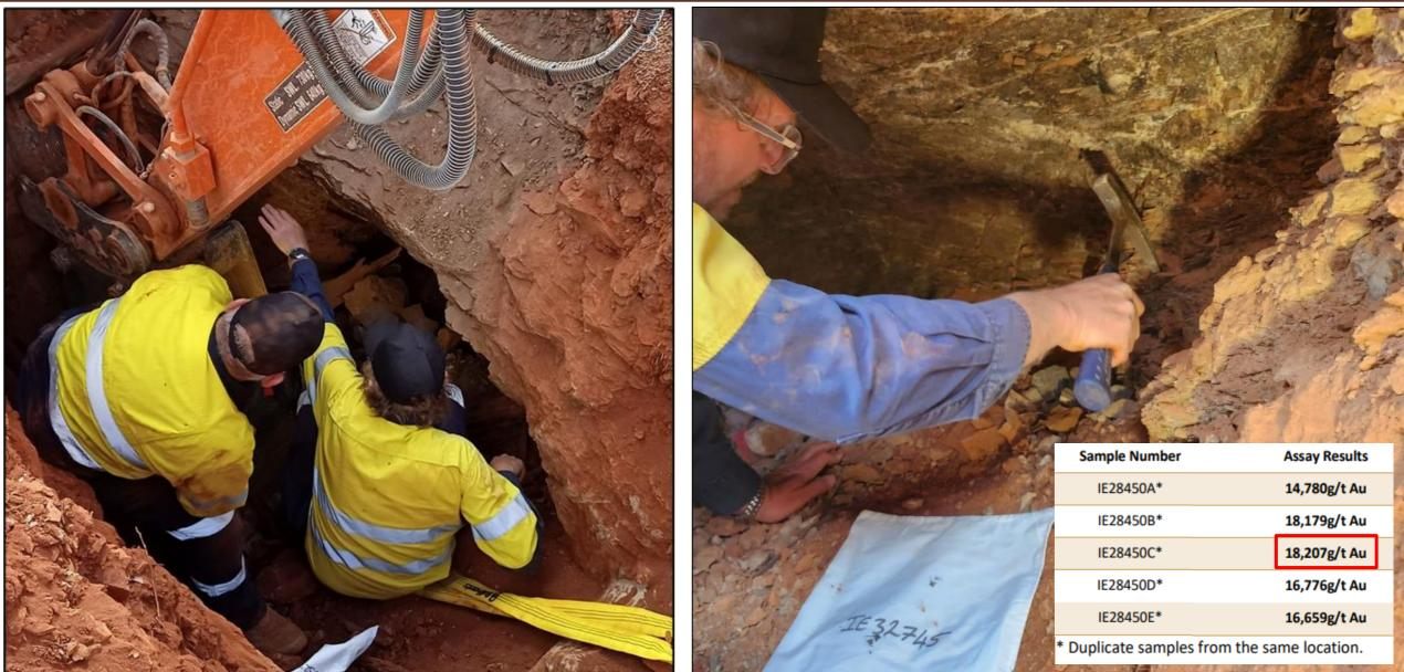
Observing geometry of the UG vein visible in the historic workings and sampling in-situ mineralisation.
