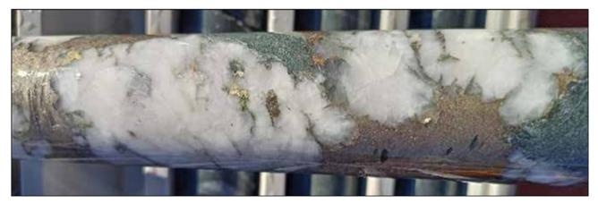
Figure 11: FMDD0047 ~231m, sulphide bearing quartz vein with pyrrhotite, pyrite, arsenopyrite and chalcopyrite hosted within andesite volcanics.
