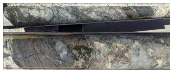
Figure 21: FMDD0032 ~116m Sulphide bearing lode structure.
