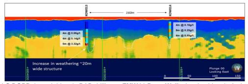
Figure 3: N-S DGPR through historic RAB drilling at FMW44-Deep Well, showing historic Au intercepts.
