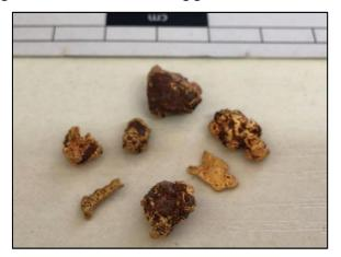
**Figure 12:** Selection of gold nuggets recovered recently in conjunction with rock chip sampling along the Northern Reflector structure. The nuggets are interpreted to be close to source due to preservation of surface textures and the presence of retained gangue mineral phases.
