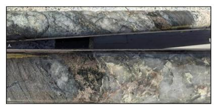
Figure 6: Lode structure at Everleigh Well ~116m in drillhole FMDD0032.
