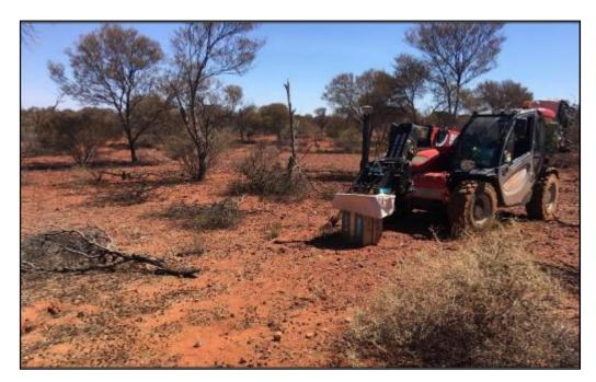
**Figure 15**: Ultramag eVibe Synchro in the field at Everleigh. The device is small and manoeuvrable, thereby greatly reducing the environmental impact of the survey. The system uses an electrical energy source that eliminates the need for the use of explosives that would have been used for a conventional seismic survey.
