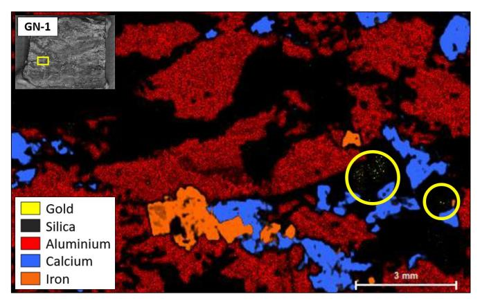
Figure 3 Micro-XRF element map of sample GN-1. Clusters of microscopic gold particles have been circled\*.
