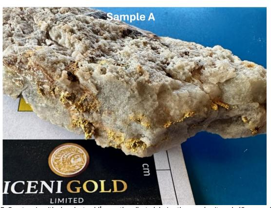
**Figure 7:** Quartz vein with abundant gold\* recently collected during the sample pit work. (Company library sample)
