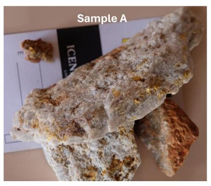
**Figure 5:** Recently collected gold\* bearing quartz veinlet. (Company library sample A)
