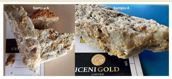
**Figure 1** Selection of gold\* bearing quartz vein samples collected from the sample trench over the Christmas Gift shear.
