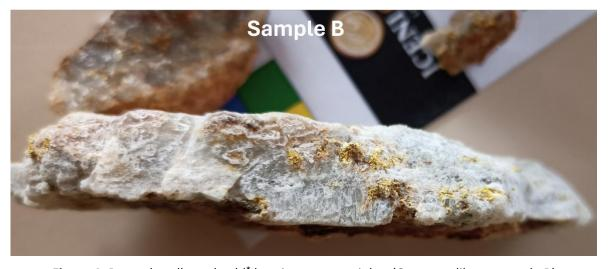
**Figure 4:** Recently collected gold\* bearing quartz veinlet. (Company library sample B)
