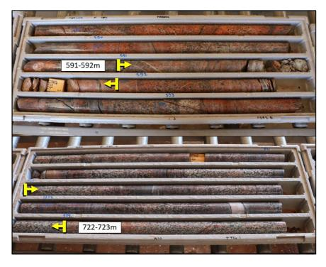
**Figure 1:** Gold mineralised intervals within FMDD0032, both intervals are hosted by altered Danjo Monzogranite with gold mineralised quartz veins and associated sulphide rich selvedges.
