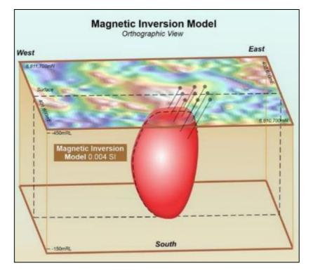
Figure 7: Schematic orthographic view of the Recon 1 magnetic anomaly and magnetic inversion model.
