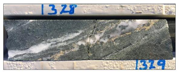
**Figure 3:** FMDD0042 ~328m, sulphide bearing quartz carbonate vein with pyrite. The alteration selvedge is carbonate and magnetite altered andesite.
