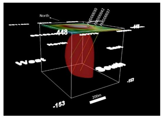
**Figure 10:** Orthographic view of the **Recon 1** magnetic anomaly and magnetic inversion model showing DD holes FMDD0030, 42 and 47 piercing the modelled magnetic body.
