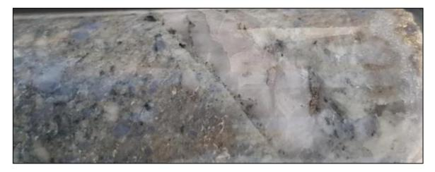
Figure 14: FMDD0042 ~66m Arsenopyrite and pyrite bearing quartz vein within altered felsic porphyry.
