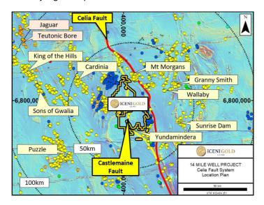
**Figure 4:** The **Celia Fault** zone passes along the eastern margin of the 14 Mile Well project while a fault splay, the **Castlemaine Fault**, passes through the centre of the project. Drillhole **FMDD0034** was designed to test adjacent to the **Castlemaine Fault** in the **Everleigh Well** target area.
