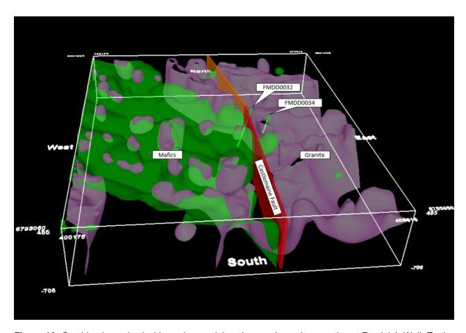
**Figure 10:** Combined geophysical inversion models using gravity and magnetics at Everleigh Well. To the west the area is dominated by higher density rocks (gravity modelled in green) interpreted as mafics. To the east the area is dominated by more magnetic rocks (magnetics modelled in pink) interpreted as granites. The position, orientation and width of the Castlemaine Fault is now constrained by the intersection in the drilling.
