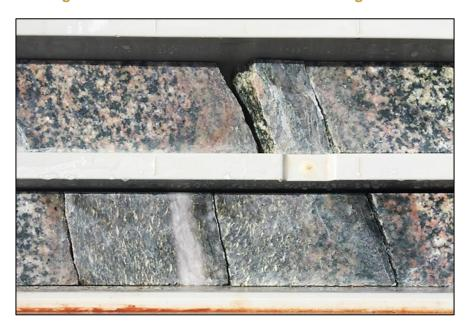
**Figure 1:** Gold mineralised intervals within **FMDD0034**, intervals are hosted within altered Danjo Monzogranite, quartz veins have very strongly altered sulphidic selvedges containing leucoxene. The hole is located immediately east of the Castlemaine Fault within a possible structural corridor or zone of influence around this structure that is favourable for the development of gold mineralised veins.
