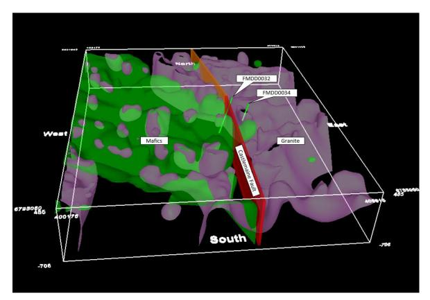
**Figure 13:** Combined geophysical inversion models using gravity and magnetics at Everleigh Well. To the west the area is dominated by higher density rocks (gravity modelled in green) interpreted as mafic. To the east the area is dominated by more magnetic rocks (magnetics modelled in pink) interpreted as granite. The position, orientation and width of the Castlemaine Fault is now constrained by the intersection in the drilling.
