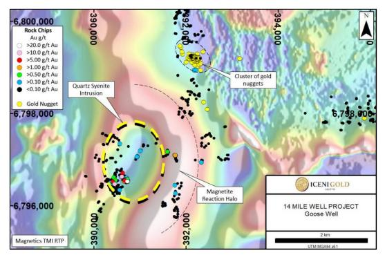
**Figure 22:** Gold anomalism in surface rock chip sampling at Goose Well, where the high-grade gold is associated with sulphide bearing quartz veins. Background image is TMI RTP magnetics.
