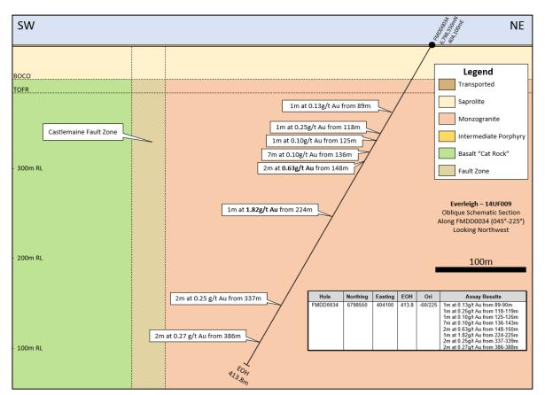
Figure 8: Schematic oblique section along the trace of FMDD0034 with the recent gold assay results.
