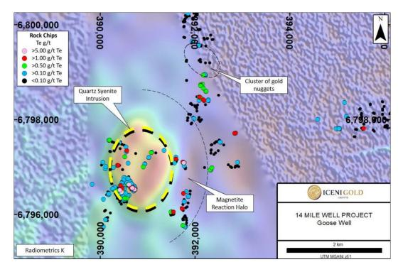
**Figure 25:** Radiometrics (K-channel) displaying the central potassium high related to the quartz syenite intrusion. Tellurium rock chip geochemistry is strongly associated with gold anomalism in and around this intrusion.
