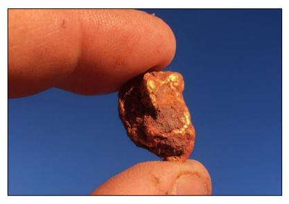
Figure 15: Gold specimen discovered at Everleigh weighing 11.2g, hosted by transported alluvium.
