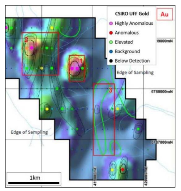
**Figure 28:** UFF+ gold soil anomaly Hage's Bore – 14UF017 is associated with a syenite related intrusion and coincident with Rare Earth Element (REE) anomalism, located 3kms east of the Guyer gold nugget anomaly.
