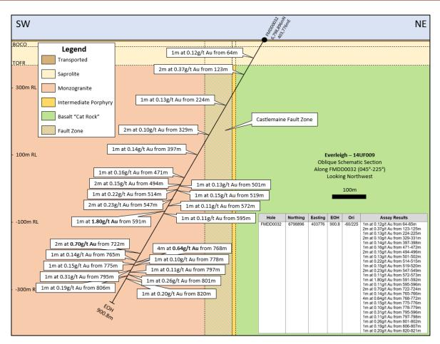
Figure 7: Schematic oblique section along the trace of FMDD0032 with the recent gold assay results.
