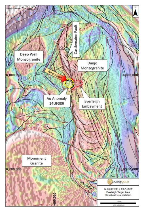
**Figure 4:** Structures in the Everleigh Well target area and the Everleigh Embayment on the margin of the Danjo Batholith. Historic work identified alteration vectoring towards the embayment. Background image is TMI RTP magnetics with a structural interpretation overlay.
