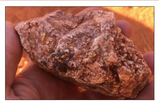
**Figure 14:** Specimen stone EV-1, ~350g, discovered at Everleigh, estimated (using the SG method) to contain 10g of gold. The gold is hosted within a quartz vein and is associated with iron oxides after sulphides (interpreted to be pyrite).
