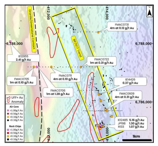
**Figure 17:** Gold results from rock chip and AC drilling at Guyer Central. The gold is associated with the Granite-Greenstone contact and a BIF unit.
