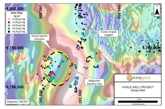
**Figure 23:** Coincident multi-element (silver) anomalism in the rock chip geochemistry at Goose Well. The target area displays a gold-silver-tellurium-bismuth metal signature, centred on and around a syenite related intrusion.
