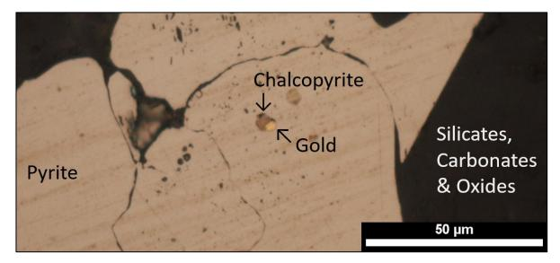
Figure 3: Photomicrograph of gold intergrown with sulphides at 224.6m in hole FMDD0032.
