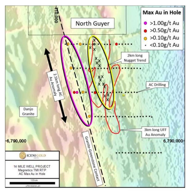
**Figure 16:** Maximum gold in hole results from AC drilling at Guyer North. The gold is associated with the eastern contact of the Danjo Granite.
