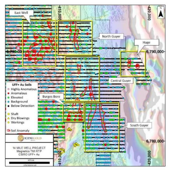
**Figure 26:** Gold anomalism in UFF+ sampling across the Guyer Well target area. The Burges Bore – 14UF016 anomaly is located on the southern edge of the project while the Hages Bore – 14UF017 anomaly is located to the east of the main Guyer trend. Background image is TMI RTP magnetics
