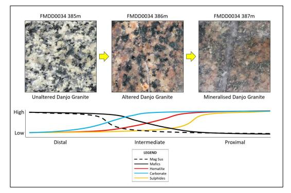
**Figure 9:** Alteration pattern observed within the Danjo Granite, where mineralisation is easily seen displaying strong hematite staining caused by the breakdown of magnetite and mafic minerals as they are converted to hematite and sulphides associated with gold mineralisation.
