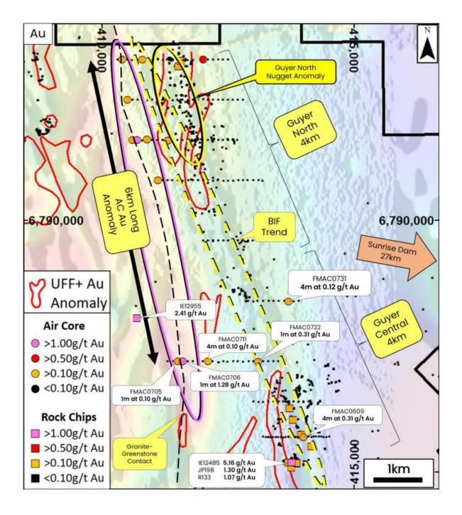
**Figure 18:** Gold results from rock chip and AC drilling at Guyer North and Guyer Central. Gold anomalism has been identified along the Granite-Greenstone contact in broad spaced drilling over a length of 6kms. Gold, silver, antimony, bismuth and tellurium anomalism is associated with a BIF unit adjacent to the Granite-Greenstone contact. This multi-element signature is similar to mineralisation at Sunrise Dam. Background image is TMI RTP magnetics.
