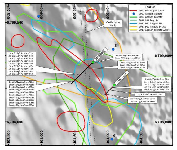
**Figure 6:** Collar plan showing the location of the DD holes and the targets identified in this area. The UFF+ gold soil anomaly is shown in red.
