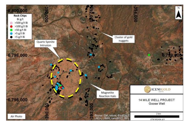
**Figure 24:** Aerial view of the syenite intrusion, which displays a distinctive circular vegetation anomaly. The Goose Well target area is located on the western boundary of the 14 Mile Well project. The geology is dominated by a quartz syenite intrusion with a prominent magnetite reaction halo.
