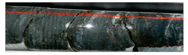
**Figure 7:** FMDD0030 ~93m Possible gold related alteration with several % pyrrhotite in biotite-chlorite altered andesite.
