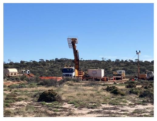
**Figure 3** Diamond drill rig operating on hole GUYDD0005, drilling west toward the Guyer Ridge in the background.
