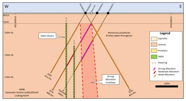
**Figure 2**: Schematic section 6,806,850mN, looking north. Two ranging drill holes identified that the strong alteration zone previously intersected is currently interpreted to be vertical. This geometry will guide further diamond drilling along strike and down dip.
