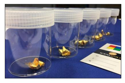
Figure 8: Gold recovered after fire assaying the high-grade Christmas Gift vein samples; these samples returned 18,207g/t Au, 18,179g/t Au, 16,776g/t Au, 16,659g/t Au and 14,780g/t Au (in ASX release dated 8 June 2023).
