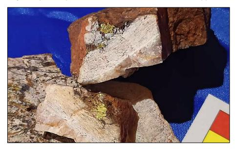
Figure 13: Gold in angular quartz fragments, at EV-5. Gold fineness measured by pXRF at 90.8-96.1% Au.
