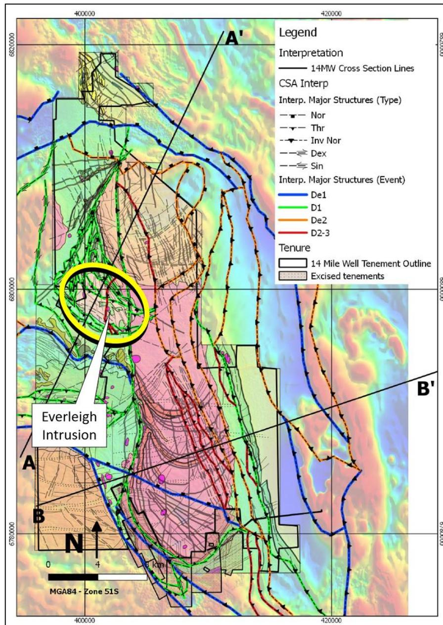
**Figure 6** Structural interpretation by CSA Global of an intrusion located at the Everleigh Embayment (Wilson, Power and Moore 2018). The intrusion is seen in geophysical data and is modelled at depth in the current 3D model.
