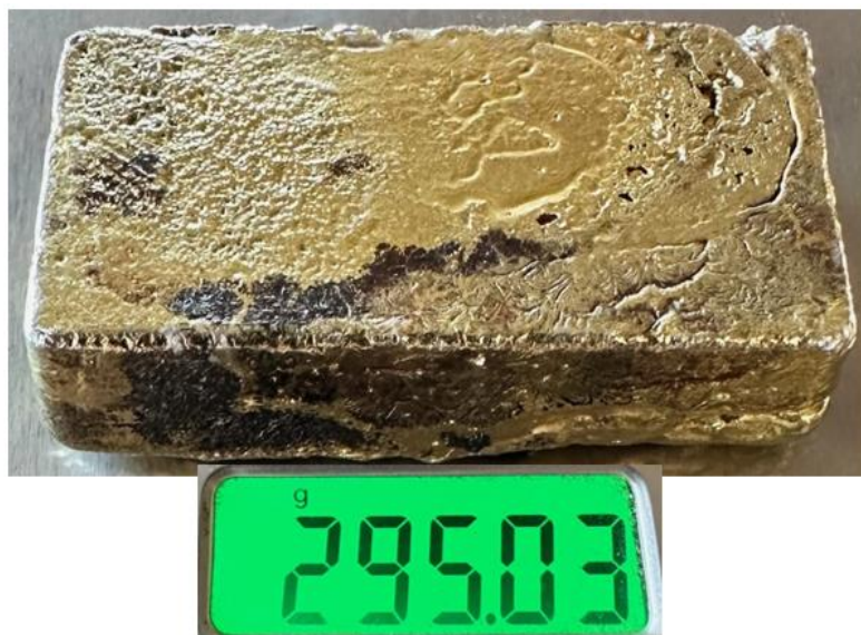
Figure 9: ~9.5oz gold doré bar* poured by the prospectors, produced from 101.3kg of Christmas Gift ore samples with a calculated grade of 2,912.4g/t**(ASX release 8 May 2024)
