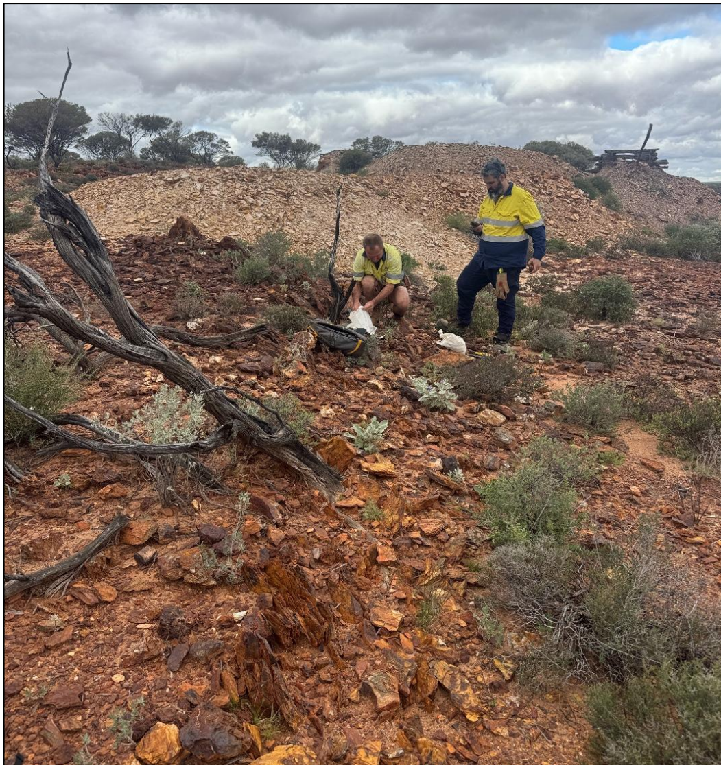
Figure 5 IcenI geologists rock chip sampling N/S trending shear zone at Rock of Ages, mullock heaps in background surrounding historic shafts.
