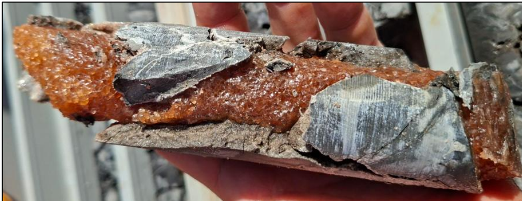
Figure 8 Example of brecciated zone from WCD001B at 1388.6m. The pink-orange coloured rock is halite (NaCl) or rock salt and represents approximately 50% of the core in this photo, remaining grey coloured rock is mudstone (ICL ASX release 29 January 2026).
