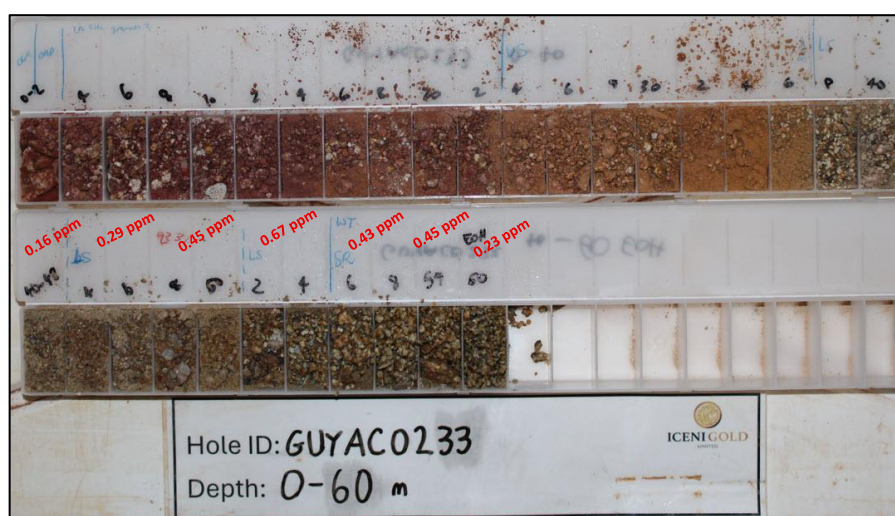
Figure 5 Chip tray photograph displaying the transported cover and end of hole geology for program's best intercept of 20m @ 0.39g/t Au from 40m to EOH (60m) in hole GUYAC0233.
