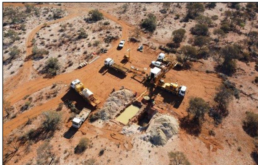
**Figure 1: Danjo NE** - Diamond Drill rig on the drill pad for hole FMDD0025. The outcropping Danjo NE quartz reef is visible in the upper left side of the image. The image is looking towards the southwest.
