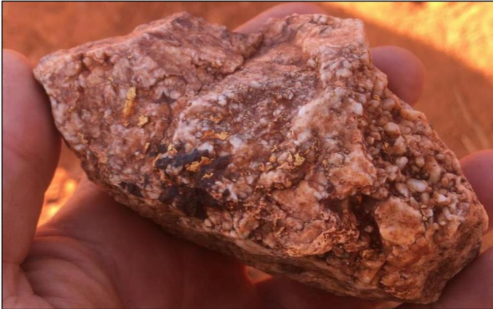
**Figure 14:** Specimen stone EV-1, ~350g, discovered at Everleigh, estimated (using the SG method) to contain 10g of gold. The gold is hosted within a quartz vein and is associated with iron oxides after sulphides (interpreted to be pyrite).
