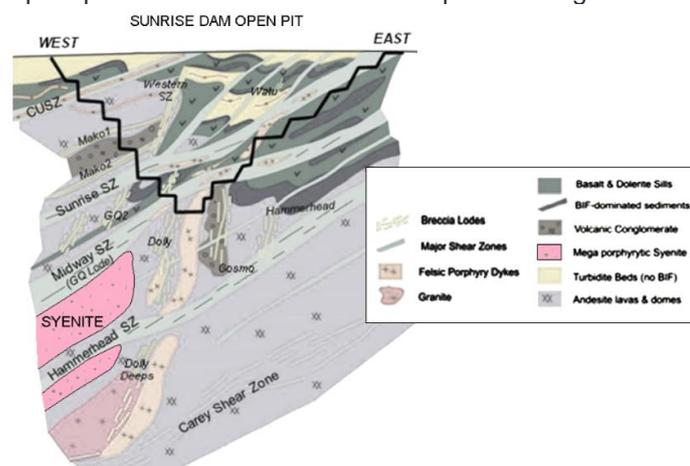
**Figure 9:** Example of the syenite and porphyries at Sunrise Dam. The image shows the relationship between the syenite, alteration and mineralised structures in the Sunrise Dam mineralised system within the Laverton District (after Nugus et al 2014).
