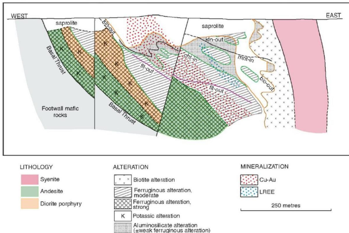
**Figure 9:** Schematic section through the Admiral Hill Gold Deposit illustrating the relationship between the gold mineralised structures and the syenite intrusion (after Witt 2018).
