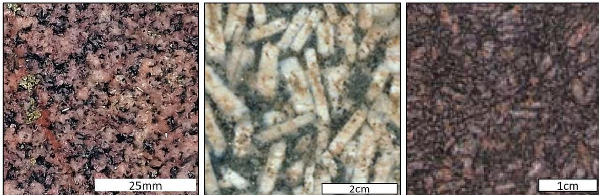
**Figure 4:** Examples of syenite intrusions. The image on the left is the altered and pyritic syenite recently identified at Deep Well. The central image is the syenite from the Wallaby Gold Deposit (after Mueller et al 2008). The image on the right is the syenite from the Karari Gold Deposit (after Witt 2018).
