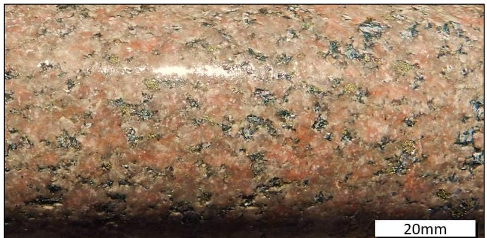
**Figure 1: TOTK** – Mineralised Syenite from 273m in FMDD0016, at TOTK. The specimen hosts brassy yellow cubic pyrite throughout (after Witt 2021).
