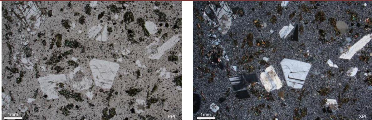
**Figure 12:** Photomicrograph of the Andesite porphyry intersected in FMDD0012. The unit displays a strong porphyritic texture. The image on the left is under plain polarised light, while the image on the right is under crossed polarised light (after Verbeeten 2021).
