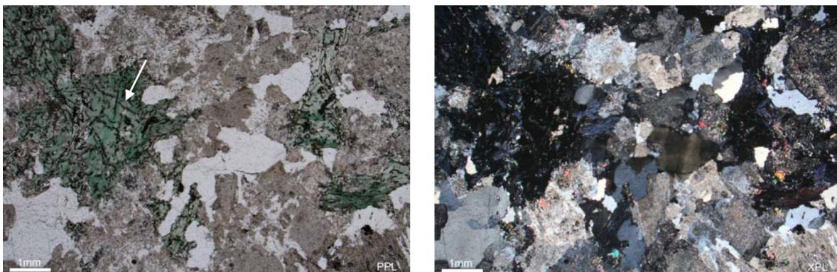
**Figure 11:** Photomicrographs of the Danjo Monzogranite intersected in FMDD0012. The unit displays a medium to coarse-grained texture. The image on the left is under plain polarised light, the image on the right is under crossed polarised light (after Verbeeten 2021).
