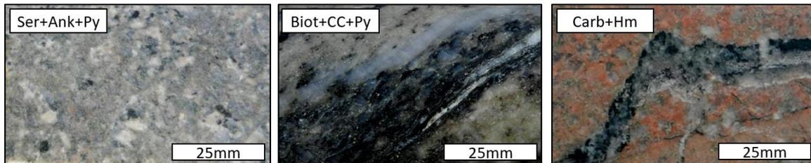
**Figure 10:** Examples of the major styles of alteration identified by Dr Witt in the diamond drill core from TOTK. The image on the left has been sericite, ankerite and pyrite altered. The central image displays biotite, calcite and pyrite alteration. The image on the right has been carbonate and hematite altered (after Witt 2021).
