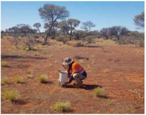
Figure 1 Haines Survey setting up a station to acquire gravity data.
