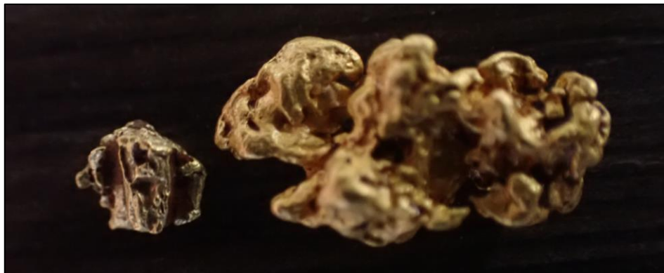
Figure 3: Types of gold recovered at Guyer. The nugget on the left is angular and pale coloured, indicating a higher silver content (~85% Au and 15% Ag, analysed by pXRF), while the nugget on the right is rounded with a deep yellow colour indicating a higher gold purity (99% Au and 1% Ag, analysed by pXRF).
