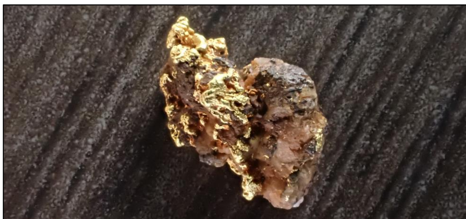
Figure 4: Angular gold from Guyer with iron oxides (after sulphides) in a quartz vein fragment.
