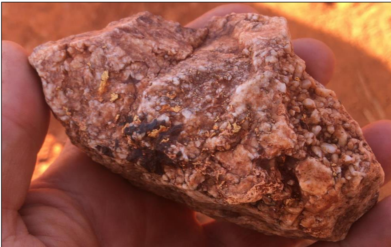
Figure 6: Specimen stone, ~350g, discovered at Everleigh, estimated (using the SG method) to contain 10g of gold. The gold is hosted within a quartz vein and is associated with iron oxides after sulphides.
