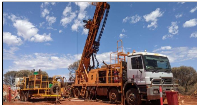
Figure 1: Diamond Drill Rig on hole FMDD0032 at the Everleigh Well Target Area, 11 January 2022.
