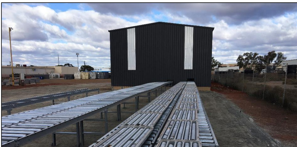
Figure 23: Roller racking at IcenI's Kalgoorlie core yard. The racks can hold 600m of NQ core, which is fed to twin Almonte diamond core saws within the shed.
