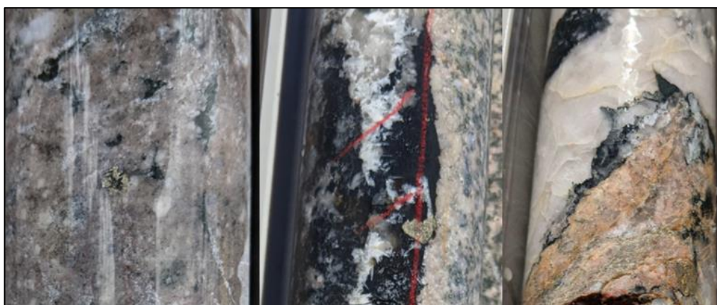
Figure 16: Examples of altered drill core from Danjo NE. Quartz veining is strongly associated with black tourmaline and silica-pyrite-white mica alteration.
