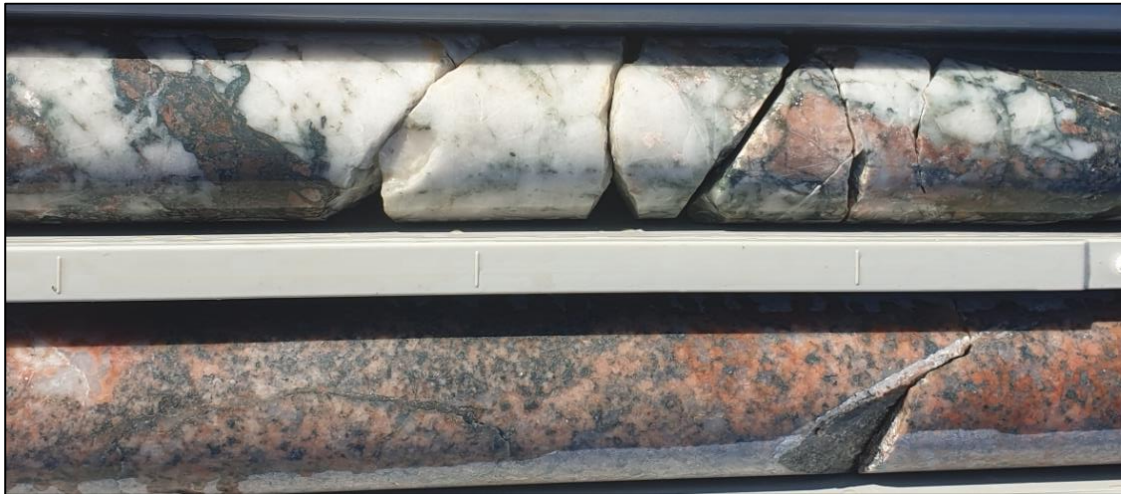
Figure 13: Strongly hematite, silica and sulphide altered drill core at ~210m in FMDD0015 at TOTK.
