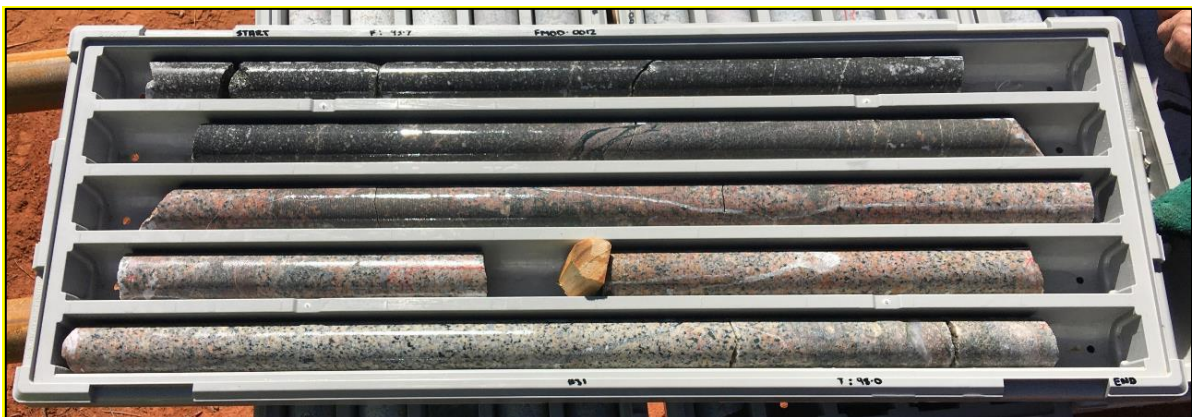
Figure 12: FMDD0012 at ~95m, showing an intermediate porphyry cutting the Danjo Granite. The porphyry contains disseminated sulphides throughout. The granite displays brecciation and hosts several quartz veins. These rocks have interacted with hydrothermal fluids that have modified significant volumes of rock. This type of alteration process is known to be associated with the formation of gold deposits.
