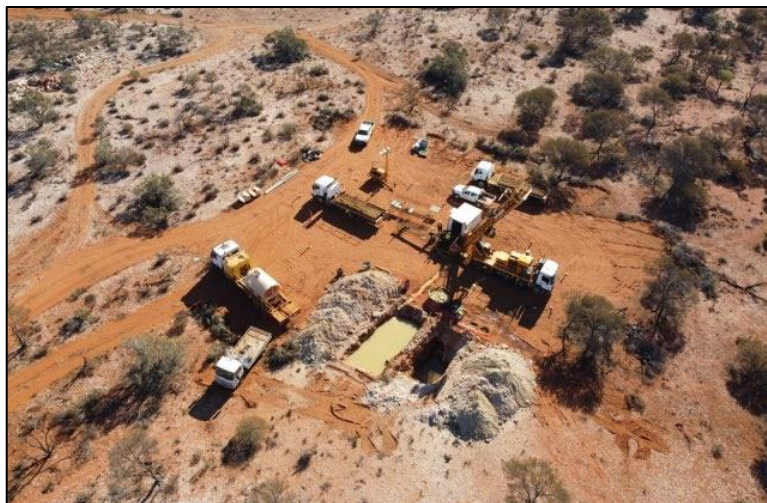
Figure 14: Danjo NE - Diamond Drill rig on hole FMDD0025. The outcropping Danjo NE quartz reef is visible in the upper left side of the image. The image is looking towards the southwest.
