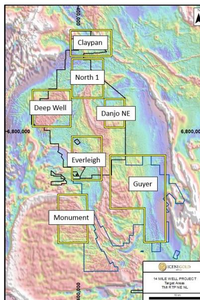
**Figure 4: 14 Mile Well project area**, showing the seven key target areas. Strong alteration has been identified across a broad area at the **Claypan** target area. DD is underway at **Claypan** and AC drilling is ongoing at **Guyer**. Image is Total Magnetic Intensity (TMI) Reduced to Pole (RTP).
