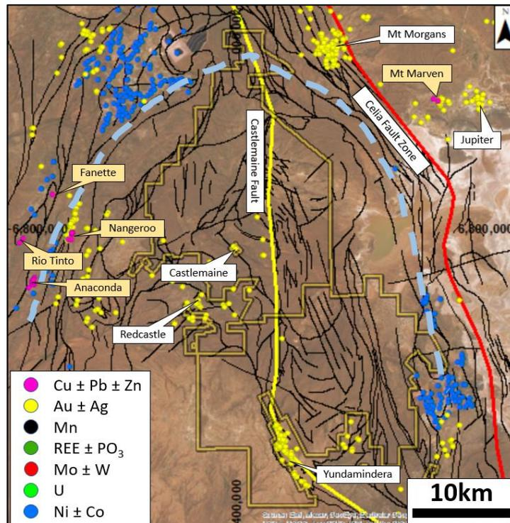
**Figure 3: Metallogenic plan of the 14 Mile Well project.** Known **VMS** mineralisation at the **Anaconda group** of mines exists immediately to the west of the **14 Mile Well project**. The underlying stratigraphy associated with this mineralisation is interpreted to extend through the **Claypan** target area (blue dashed line).
