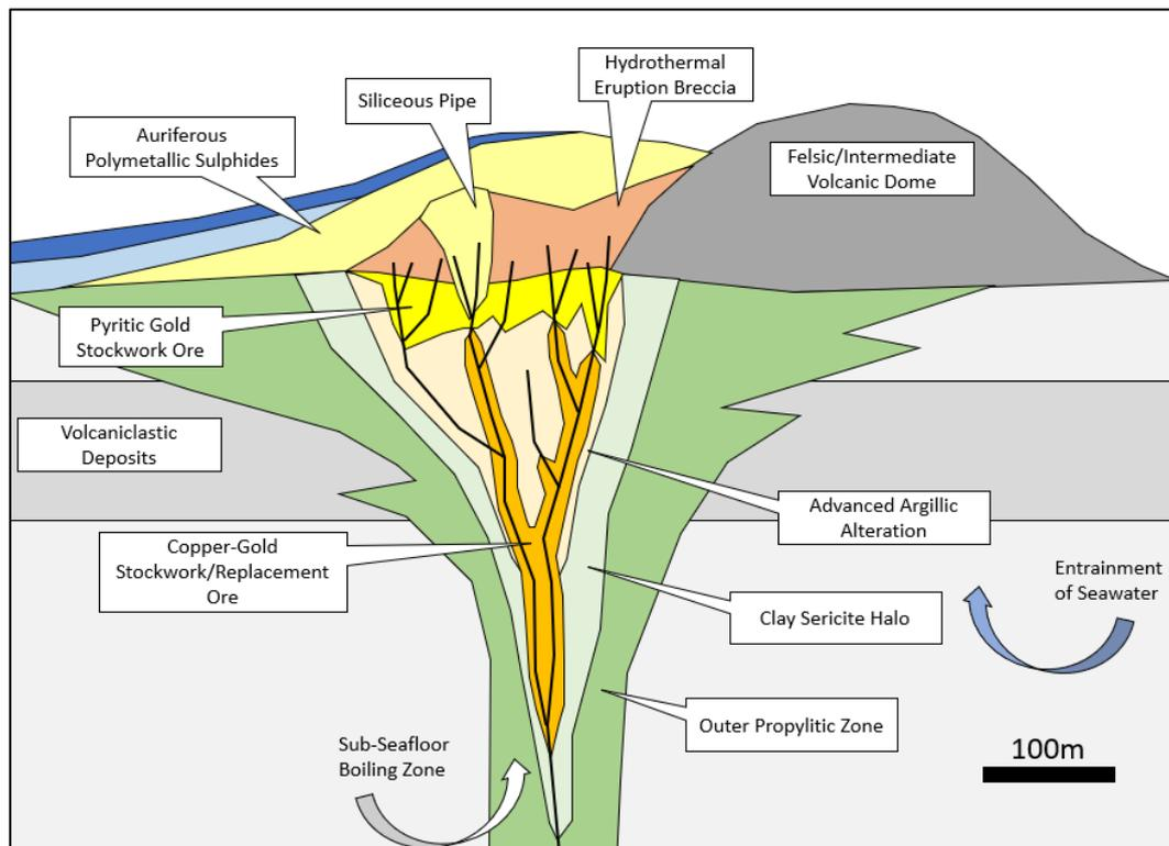
**Figure 7:** Schematic section through a gold rich **VMS hydrothermal system** (after Dube et al 2007.)
