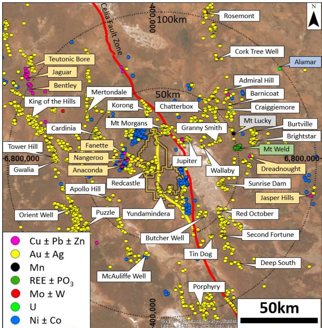
**Figure 2:** Metallogenic plan of the Laverton district. Known **VMS** mineralisation at the Anaconda group of mines exists immediately to the west of the **14 Mile Well project**. The underlying stratigraphy associated with this mineralisation is interpreted to extend through the **Claypan target area**, where the **Castlemaine Fault** and **Celia Fault** zones are interpreted to interact.
