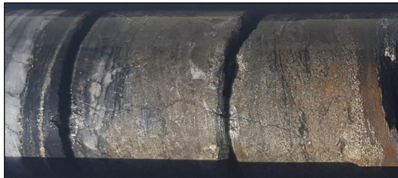
**Figure 1:** FMDD0040 ~140m, sulphide rich zone associated with BIF/chert.
