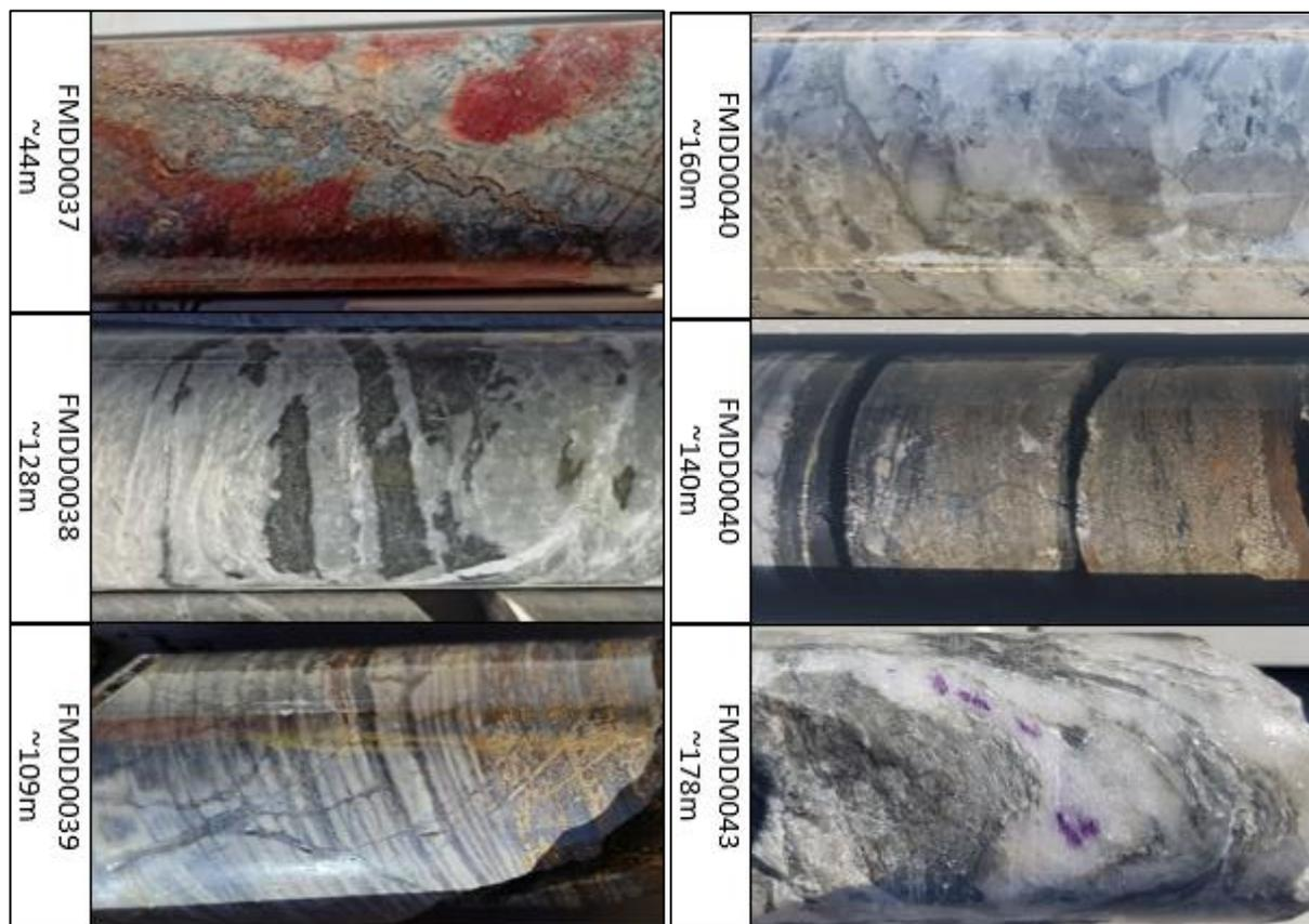
**Figure 8:** Examples of observed alteration styles in drill core from the **Claypan** target area:
