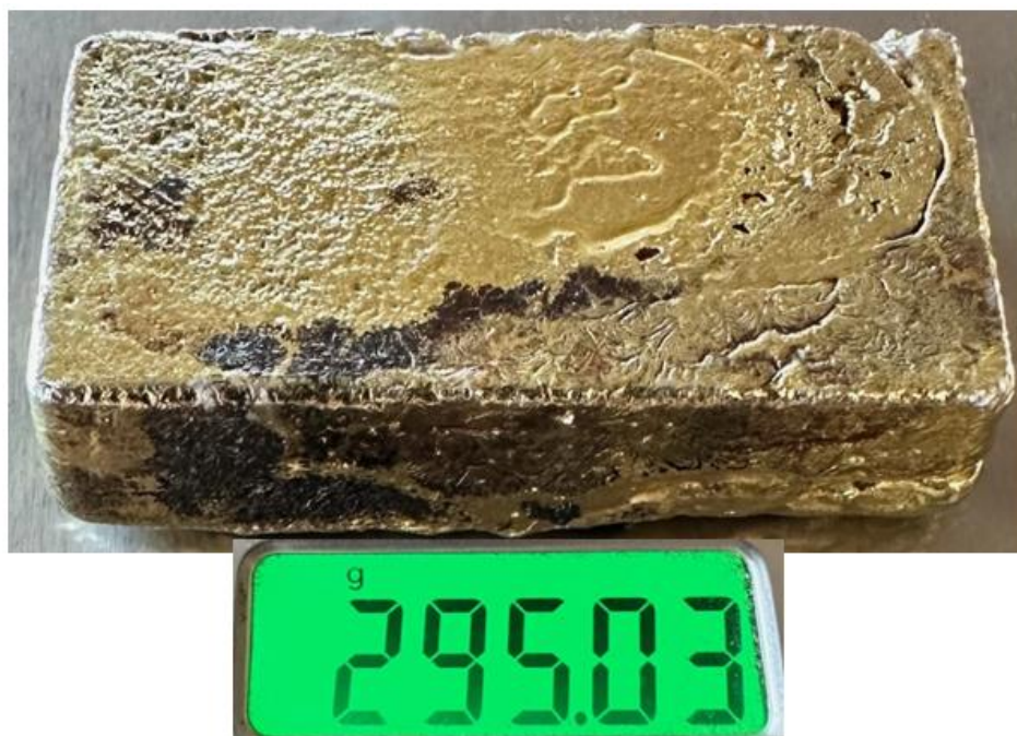
Figure 6 ~9.5oz gold doré bar* poured by the prospectors, produced from 101.3kg of Christmas Gift ore samples with a calculated grade of 2,912.4g/t**.
