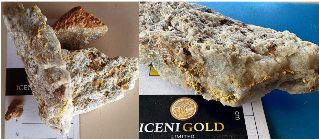
Figure 1 Selection of gold* bearing quartz vein samples collected from the sample trench over the Christmas Gift shear.
