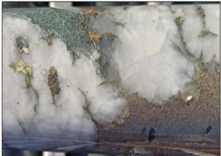
Figure 55 Drill core from FMDD0047 showing sulphide bearing quartz vein
