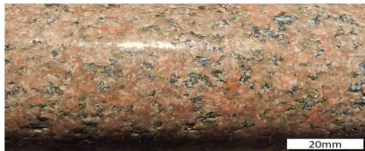
Figure 58 Drill core - Syenites with Potassic Feldspars and disseminated pyrite
