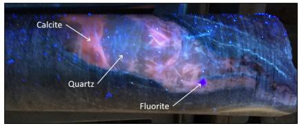
Figure 1: Claypan hole FMDD0043 ~117m: Quartz-calcite-fluorite, under ultra-violet illumination.
