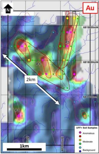
**Figure 5:** The UFF+ gold soil anomaly 14UF014 at Claypan has a priority 1 zone that is 2km long. This zone is coincident with the sub-cropping BIF unit that has been tested by the recent DD program.
