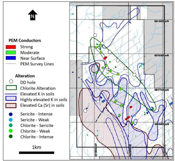
**Figure 4: Alteration patterns** identified by the current work campaign and the historical PEM conductors identified by previous explorers. The conductors may represent concentrations of sulphides that are associated with the alteration boundaries in the bi-modal rhyolite-andesite volcanic sequence. This is a geological environment that can host Au rich VMS systems.
