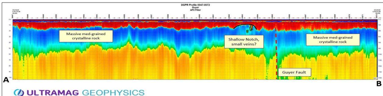
**Figure 4:** DGPR Survey line across the Guyer Fault, demonstrating the geophysical response of the structural zone. The deepening of the overlying cover sequence has been confirmed by recent AC drilling.
