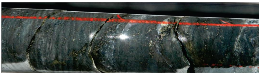
Figure 25: FMDD0030 ~93m Possible gold related alteration with several % pyrrhotite (visual estimate) in biotite-chlorite altered andesite.
