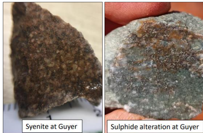
Figure 42: Examples of a favourable syenite intrusion and sulphide altered andesite intersected by AC drilling in the Guyer Target Area.
