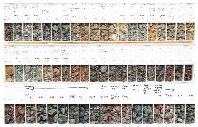
Figure 4 GUYRC0028 (180m to 238m EOH) displaying large, broad, pervasive altered zones of mineralisation with the granodiorite host rock. Numbers in red (g/t) superimposed on the chip trays are the reported gold assays grades over each representative sample interval.
