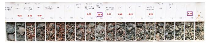
Figure 3 GUYRC00028(140m to 160m) displaying broad, pervasive hematite alteration (142m to 152m) and sericite silica altered zone (140m to 156m) in the host granodiorite. The high-grade mineralisation (149m-150m) is associated with quartz veining. Numbers in red (g/t) superimposed on the chip trays are the reported gold assays grades over each representative sample interval.
