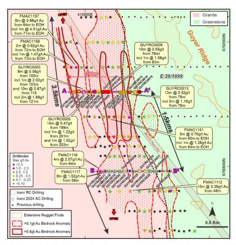
**Figure 6** Geological map and drillholes completed at Guyer North showing the 2025 RC drillholes, 2024 AC drillholes, significant gold results and the interpreted >0.1gt/t and >0.5 g/t Au bedrock gold anomalies. Refer to Figure 7 for drillhole cross-sections AA'.
