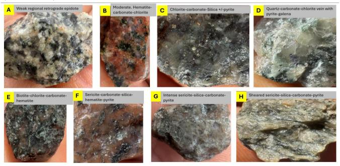
Figure 5 Selection of RC drill chips highlighting the various types of alteration in the granodiorite host rock.
