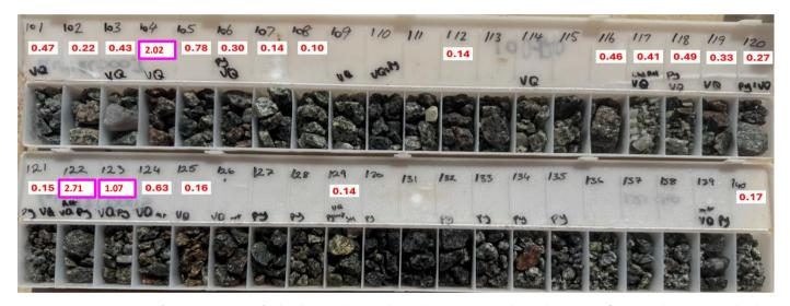
Figure 4 GUYRC0003 (100m to 140m) displaying large, broad, pervasive altered zones of mineralisation with the granodiorite host rock. Numbers in red (g/t) superimposed on the chip trays are the reported gold assays grades over each representative sample interval.
