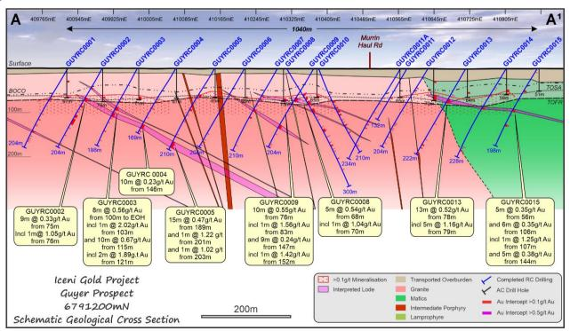
**Figure 7** Drillhole cross-section AA' on 6791200mN displaying 16 RC holes drilled at Guyer. Significant intercepts for eight RC holes displayed. Refer to Table 1 below for full list of the significant intercepts.
