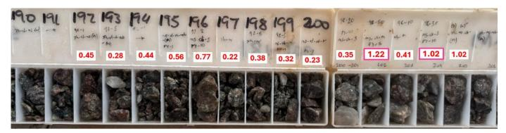
**Figure 3** GUYRC0005 (189m to 206m) displaying large, broad, pervasive hematite alteration (189m to 200m) and sericite silica altered zone (200 to 204m). Large broad zone of mineralisation 15m at 0.47g/t within the granodiorite host rock. Numbers in red (g/t) superimposed on the chip trays are the reported gold assays grades over each representative sample interval.
