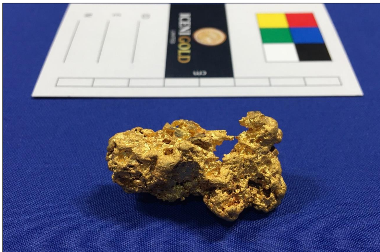
Figure 2: Nugget* GY-1 after cleaning. The nugget has a gold fineness of 99.1% (measured by pXRF) (ASX release 19 June 2023).
