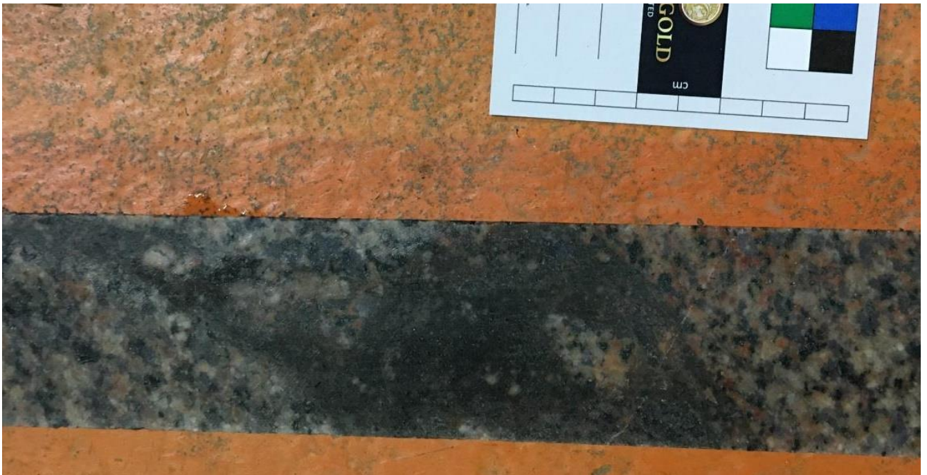
Figure 10: FMDD0012, brecciated and strongly altered Danjo Granite hosting disseminated sulphides, the sulphide concentration increases between the breccia clasts (dark coloured region), where fluid flow was the greatest. This is significant because brecciation and associated sulphide deposition are known processes in the formation of large gold deposits, these characteristics have been observed in all of the large gold mines in the Laverton District. This sample is from the ~90m thick strong alteration zone.
