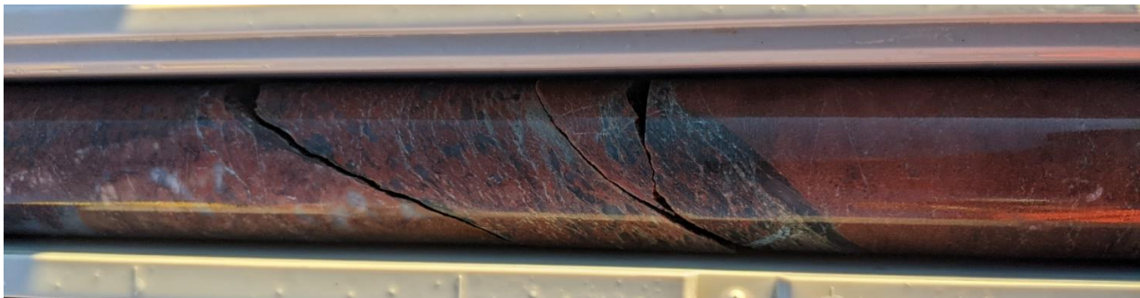
Figure 7: FMDD0012 at ~307m, intense silica hematite alteration overprinting the Danjo Granite. This is significant because the formation of hematite at the expense of other iron bearing minerals is commonly associated with the formation of gold deposits.
