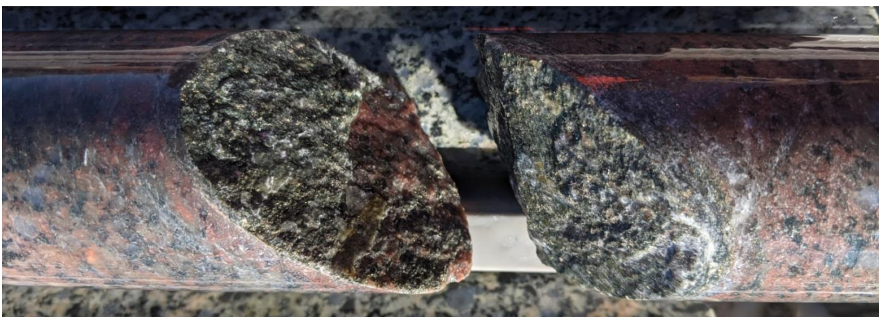
Figure 8: FMDD0012 at ~340m, strong hematite alteration zone with chlorite and disseminated sulphides.
