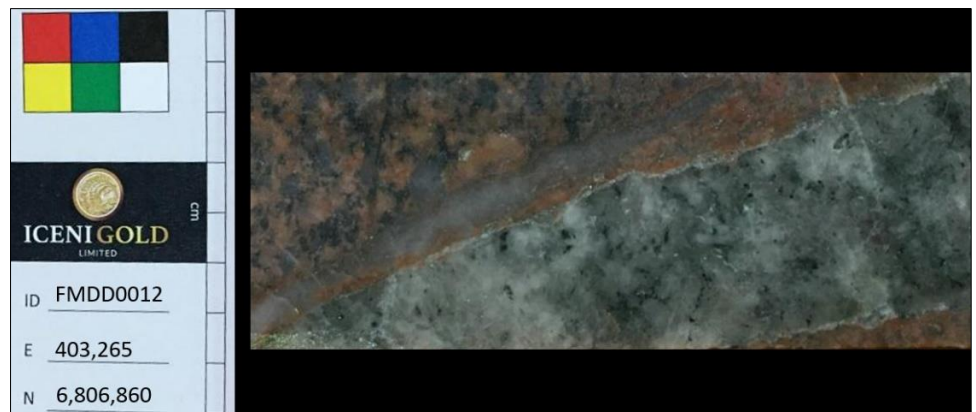
Figure 1: Strongly altered granite cut by different styles of quartz veins with associated sulphide, HQ ½ core from FMDD0012.
