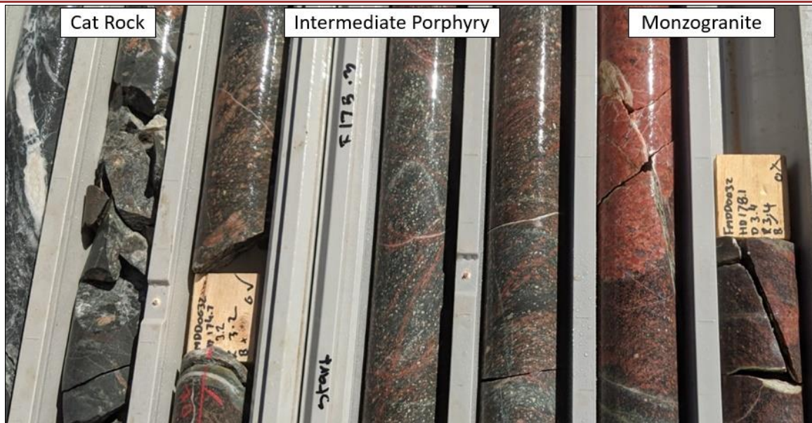
Figure 25: FMDD0032 ~ 175m Hematite-silica altered intermediate porphyry that cuts the Danjo Monzogranite and exploits the adjacent cat rock contact.
