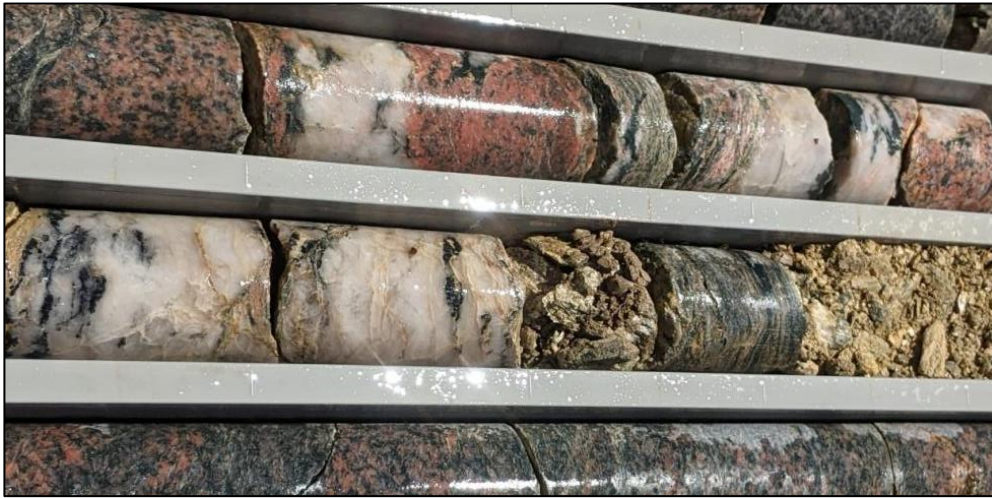
Figure 27: Alteration in FMDD0026, the Danjo Monzogranite is cut by quartz tourmaline pyrite veins with hematite, pyrite and white mica alteration.
