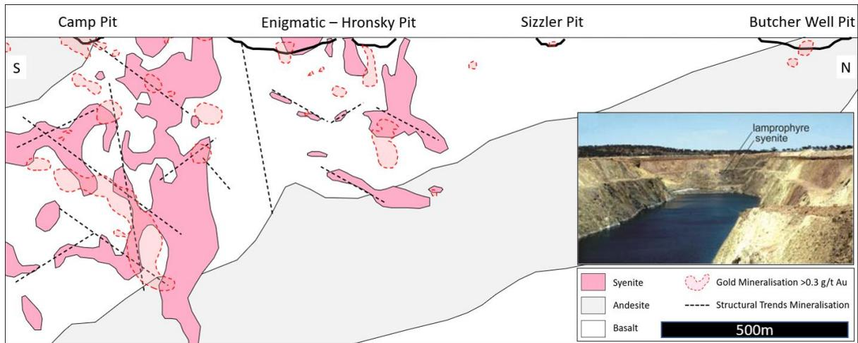
**Figure 8:** Schematic section through the Butcher Well Gold Deposit illustrating the relationship between the gold mineralised structures and the syenite intrusion (after Kent 2021). Inset image illustrates the syenite and lamprophyre exposed in the Butcher Well open pit (after Witt 2018).
