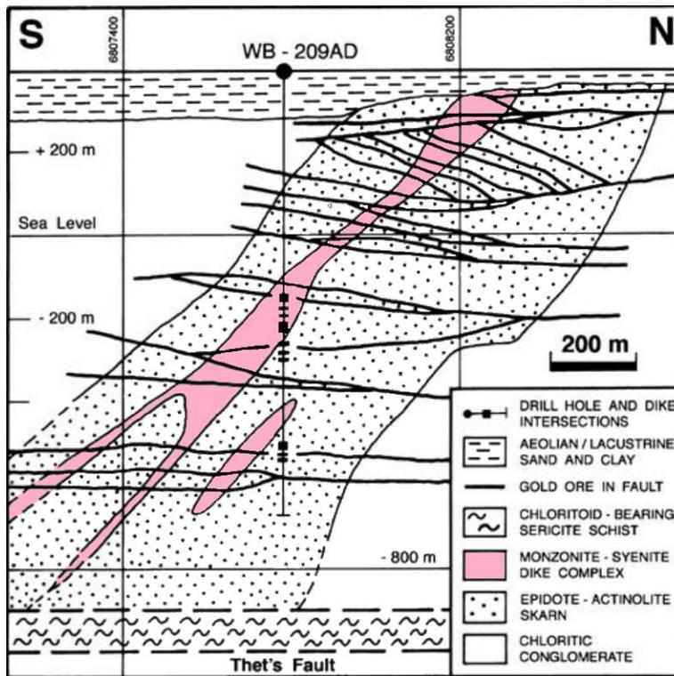
Figure 6: Schematic cross section through the Wallaby Gold Deposit illustrating the relationship between the gold mineralised structures and the syenite intrusion (after Mueller et al 2008).
