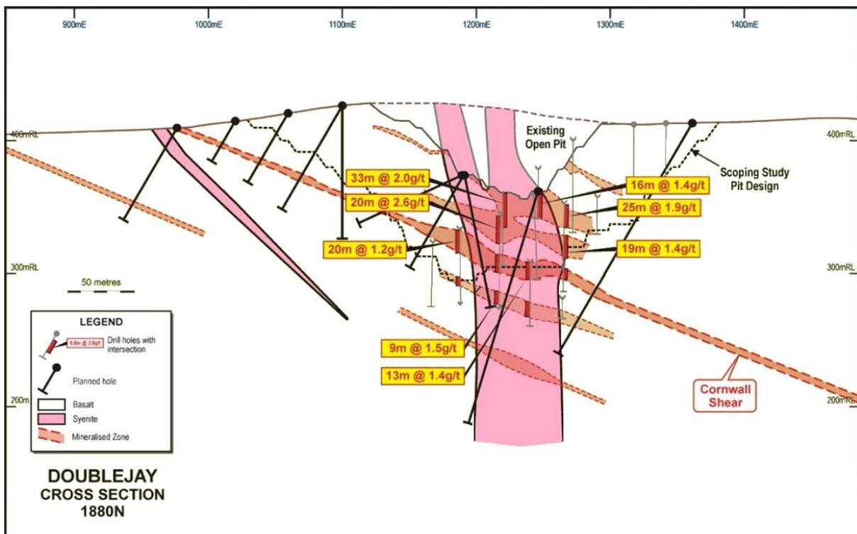
Figure 7: Schematic cross section through the Jupiter Gold Deposit illustrating the relationship between the gold mineralised structures and the syenite intrusion (after Williams 2015).
