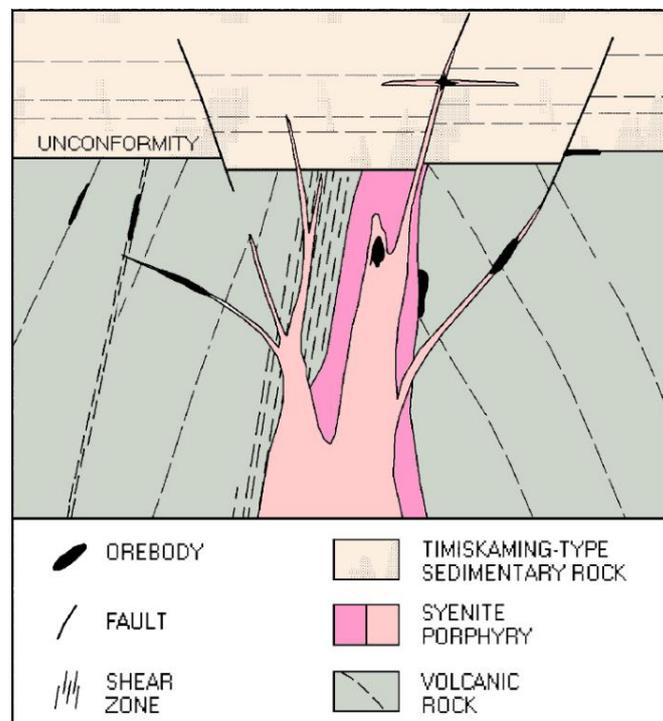
**Figure 5:** Schematic model illustrating the styles of mineralisation associated with syenite intrusions (after Robert 2001).
