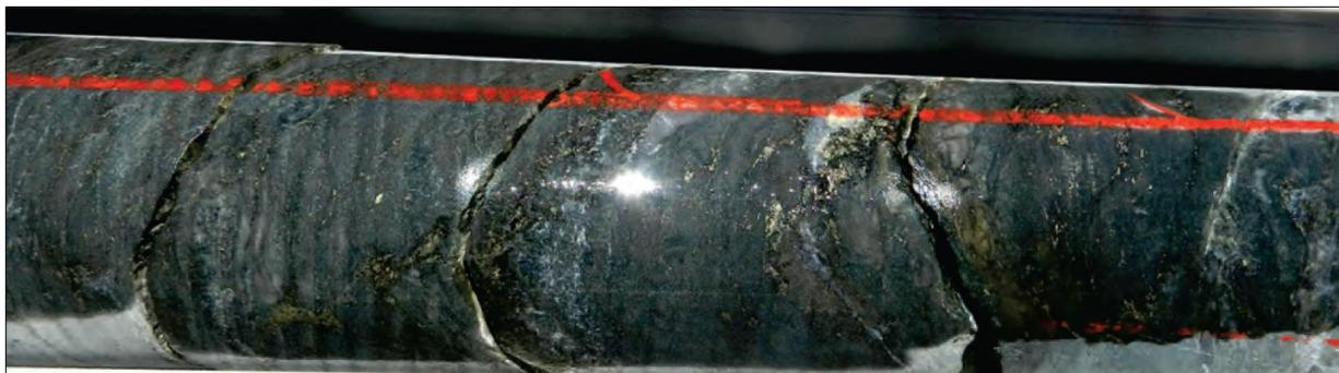
**Figure 7:** FMDD0030 ~93m Possible gold related alteration with several % pyrrhotite in biotite-chlorite altered andesite.
