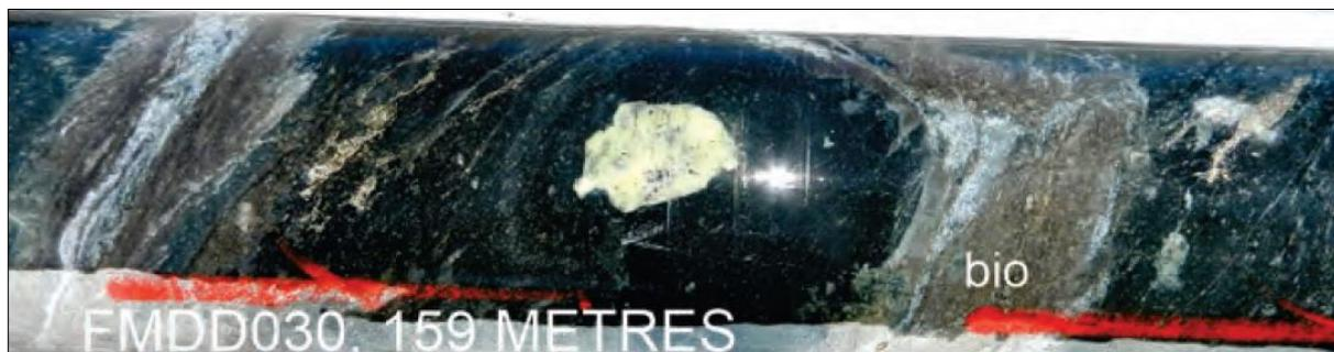
**Figure 6:** FMDD0030 ~159m Biotite dominated alteration assemblage around andesite pillow margins
