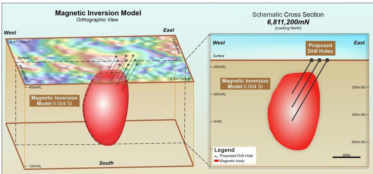
**Figure 5:** Recon1 magnetic anomaly and magnetic inversion model.
