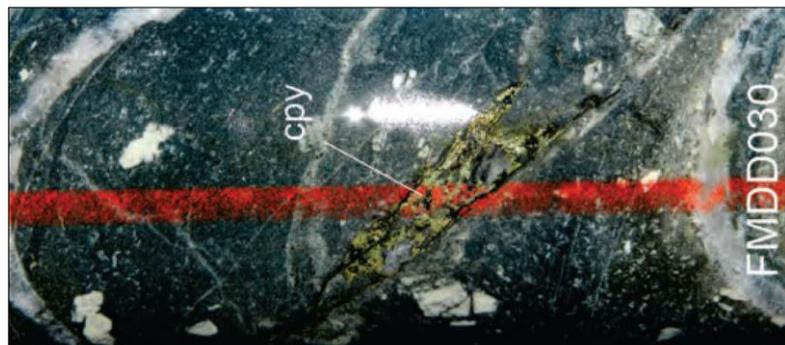
**Figure 1:** FMDD0030 ~80m, chalcopyrite veining in brecciated andesite.
