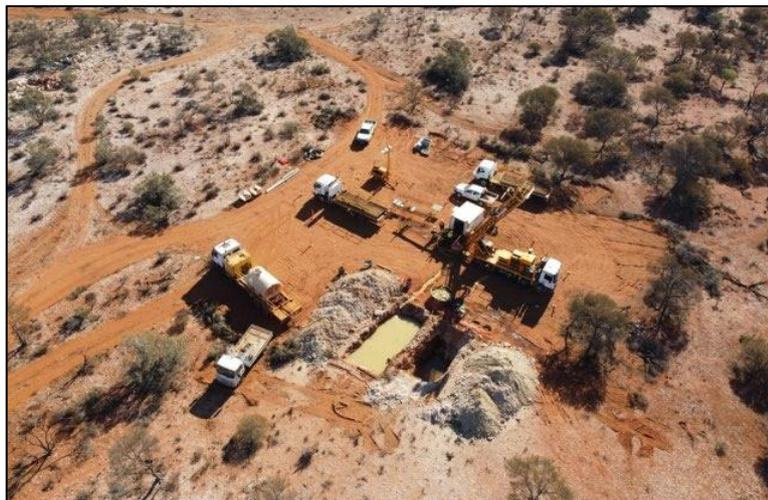
**Figure 16: Danjo NE** - Diamond Drill rig on hole FMDD0025. The outcropping Danjo NE quartz reef is visible in the upper left side of the image. The image is looking towards the southwest.
