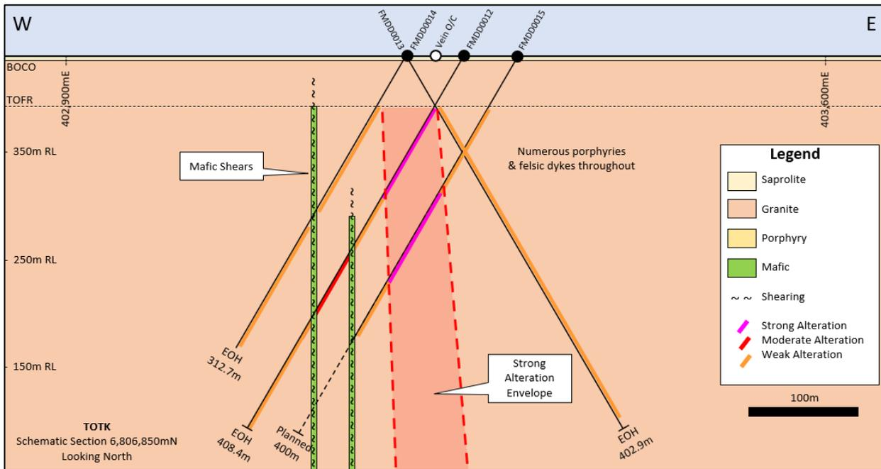
**Figure 2:** Schematic section 6,806,850mN, looking north. Two ranging drill holes identified that the strong alteration zone previously intersected is currently interpreted to be vertical. This geometry will guide further diamond drilling along strike and down dip.
